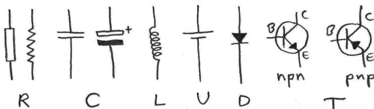
Figure 12. Symbols for resistor (R), capacitor (C), inductor (L), DC voltage source (U), diode (D), transistors (T).
