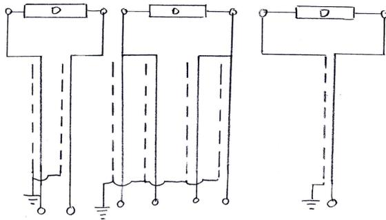
Figure 21. Simple representation of shielding principles. Left and right: Shields connected to ground in 2- and 4-wire setups, thereby acting as guards against crossover signals (capacitive and conductive). Right: A simpler setup in which the “low” (here grounded) is as a shield around the “high” conductor. This does not guard against crossover between the two (!) but merely shields against intrusion of external signals.
