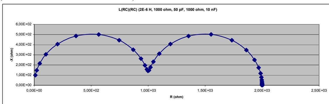
Figure 30. Nyquist impedance plot of an  $L(RC)(RC)$  circuit typical of a ceramic with bulk and ideal grain boundary contributions to the impedance.
