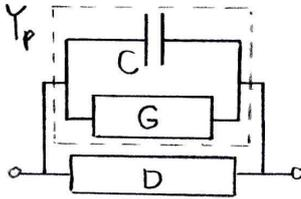
Figure 18. Parasitic admittance elements; conductance and capacitance.
