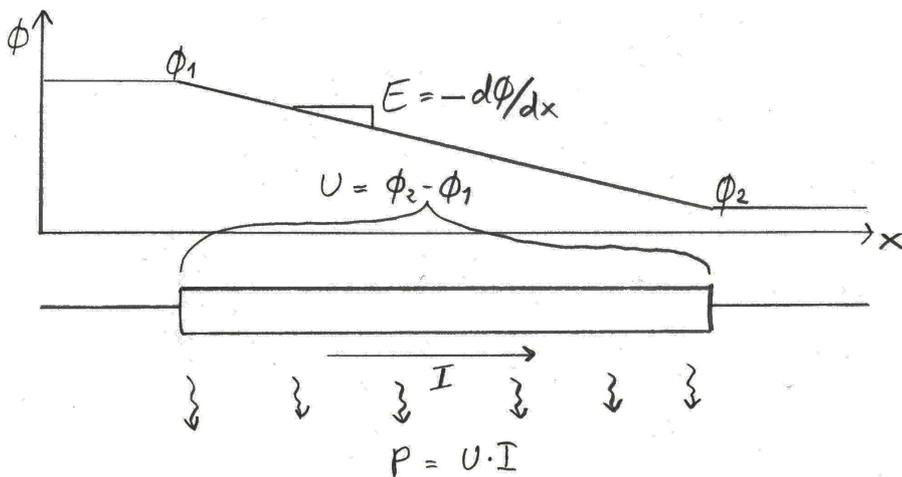
Figure 3. Schematic illustration of electrical potential, field, voltage, current, and power in relation to current passing through a resistor.
