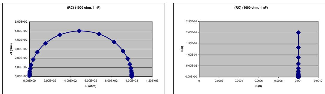
Figure 28. Nyquist-type impedance and admittance plots of a parallel circuit of one resistor and one capacitor, over a frequency range of  $10^{-5}$  to  $3 \cdot 10^7$  Hz.
