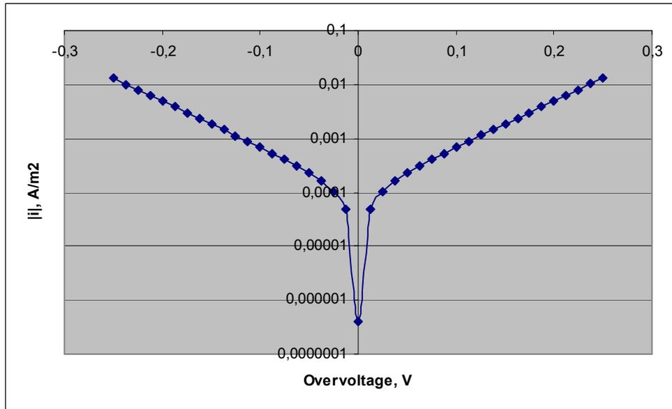
Figure 25. Tafel plot for the same parameters as in the previous plot ( $i_0 = 0.0001 \text{ A/m}^2$ )
