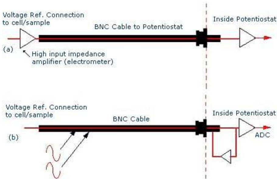
Figure 22. Two simple ways of reducing noise and losses in high impedance low level measurements. (a) A high-impedance (electrometer) preamplifier is placed close to the sample. (b) Driven shield. From Solartron.
