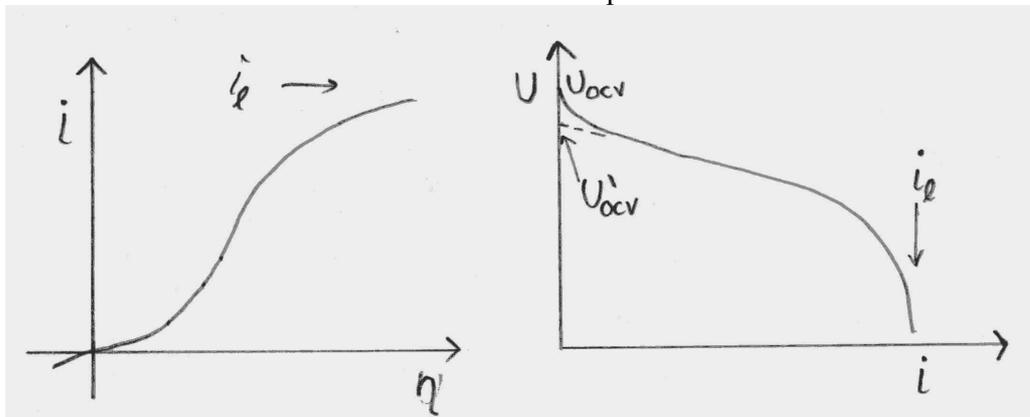
Figure 26. Plots illustrating effects of concentration polarization and mass transport limitations. Left: current density  $i$  vs overpotential. Right: Typical  $i$  vs  $U$  curve for a fuel cell: The open circuit voltage  $U_{OCV}$  falls by concentration polarization; as the electrodes get stable concentrations of products, the curve relates to a new open circuit voltage  $U'_{OCV}$ . Mass transport limiting current density is denoted  $i_l$ .
