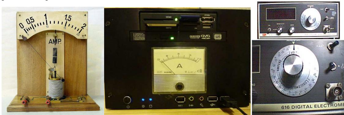
Figure 2. Three old amperemeters. The leftmost and middle have coil-driven analog pointers, while the rightmost is an electronic digital research multimeter (electrometer) from the 1980s which measures the current by the voltage over standard resistors.
