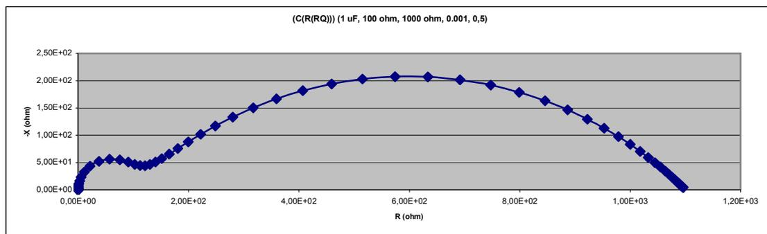
Figure 34. Nyquist plot of a Randle’s circuit for a typical poor, but not blocking electrode.
