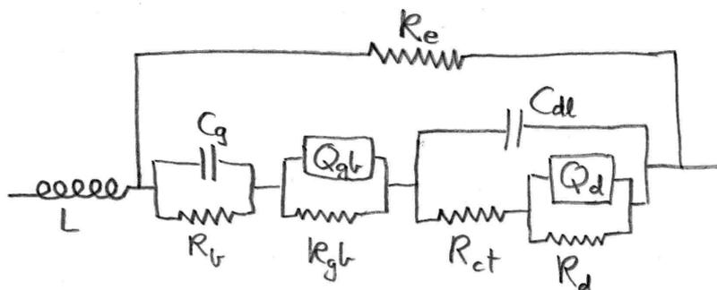
Figure 37. Equivalent circuit that may apply to a typical sample of a mixed ionic– electronic conductor. For simplicity, electronic conductivity assumed not to have grain boundary impedance.
