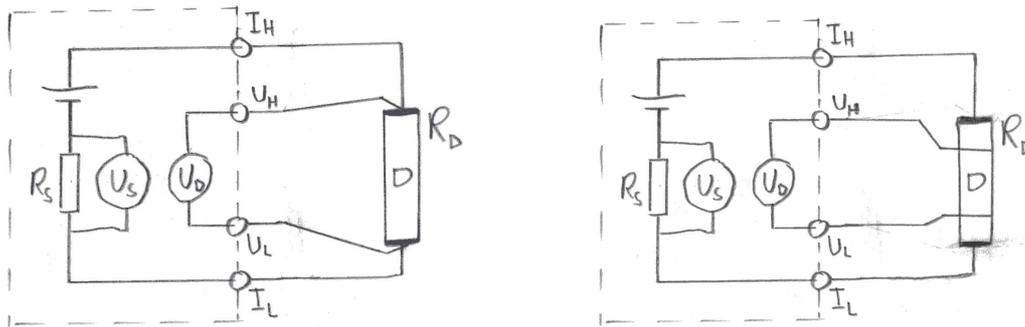
Figure 14. 4-terminal instruments used with 4 wires. Left: 2-electrode measurement (sample and electrodes). Right: 4-electrode measurement (sample material only).
