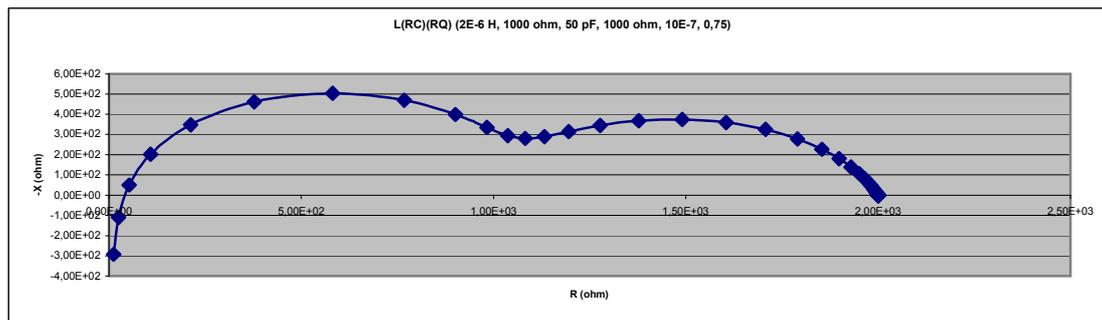
Figure 32. Nyquist impedance plot of an  $L(RC)(RQ)$  circuit typical of bulk+grain boundary impedances in a real ceramic.
