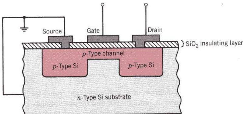
Figure 11. In this MOSFET transistor, the p.type channel is normally depleted and thus blocking because of its neighbouring n-type substrate. However, input signals to the gate charges the channel electrostatically through the thin insulating oxide layer. This opens the otherwise depleted channel and allows current to pass between source and drain.
