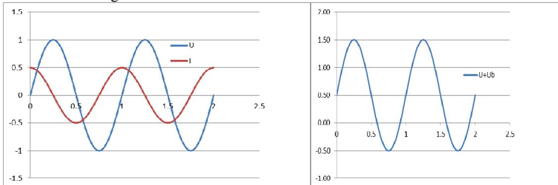
Figure 5. Left: AC voltage and current. Right: Biased AC voltage.
