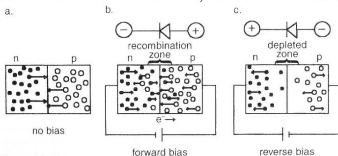
Figure 8. Illustration of a p-n junction and its conducting and blocking actions under forward and reverse bias.
