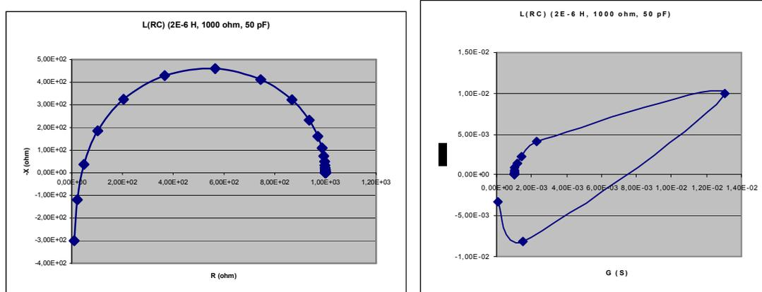
Figure 29. Nyquist impedance and admittance diagrams of the circuit  $L(RC)$  representing a bulk sample with conductance  $G=1/R$ , geometric capacitance  $C$ , and inductance  $L$  (real or parasitic). The points on the strange high frequency part of the curve in the admittance plot is in fact part of a circle.
