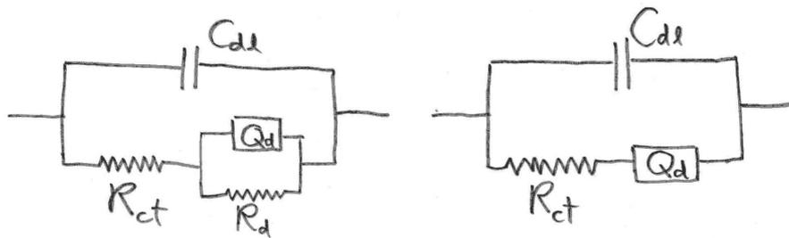
Figure 33. Typical equivalent circuits for non-blocking (left) and blocking (right) electrodes.
