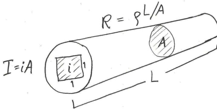
Figure 4. Schematic illustration of terms relating to current and resistance
