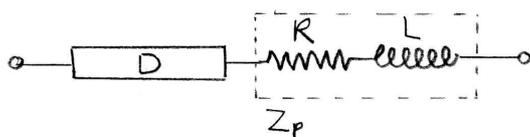
Figure 17. Parasitic impedance elements; resistance and inductance.
