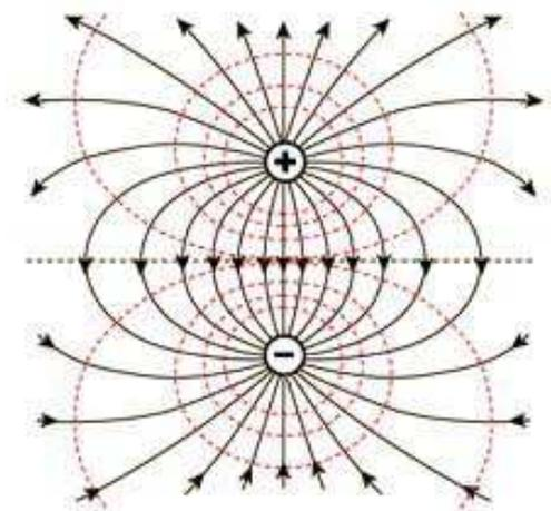
**Voltage,  $U$** , is the difference in **electrical potential,  $\phi$**  between two locations:  $U = \Delta\phi = \phi_2 - \phi_1$ . The unit for voltage  $U$  is V (volt).
