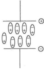
Figure 6. Depolarisation of a capacitor by dipoles in the dielectric.
