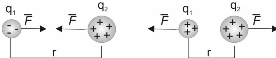
Figure 1. Electrical charges are multiples of positive or negative elementary charges, Objects of opposite or the same sign of net charge attract or reject each other, respectively.
