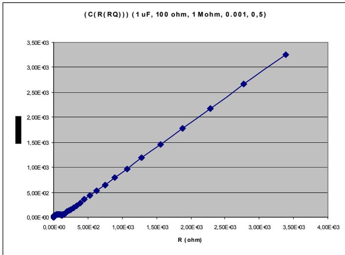
Figure 35. Nyquist plot of a Randle's circuit for a typical almost blocking electrode ( $C_{dl}(R_{ct}(R_dQ_d))$ ), with  $R_d = 1$  Mohm. Lowest frequencies omitted for clarity of illustration. Circuit effectively corresponds to  $(C_{dl}(R_{ct}W_d))$ .
