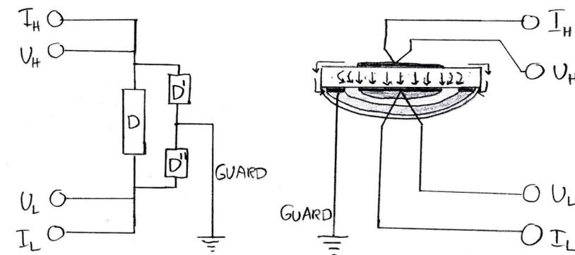
Figure 20. Guarded measurements to obtain the impedance of an element  $D$  in a circuit including other elements  $D'$  and  $D''$  (left) and to eliminate the surface conduction of a solid sample using a ring electrode on a disk (right). Arrows in the latter indicate currents.
