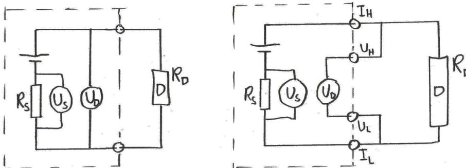
Figure 13. Schematic principle of resistance measurements using 2 electrodes and 2 wires. Left: 2-terminal instrument (typical handheld). Right: 4-terminal instrument. In both cases the wires to the device (D) contribute to the voltage drop and thus to the resistance. The terminology  $I_H$ ,  $U_H$ ,  $U_L$ ,  $I_L$  for the four terminals is typical, reflecting current and voltage terminals in order of going from high to low potential.
