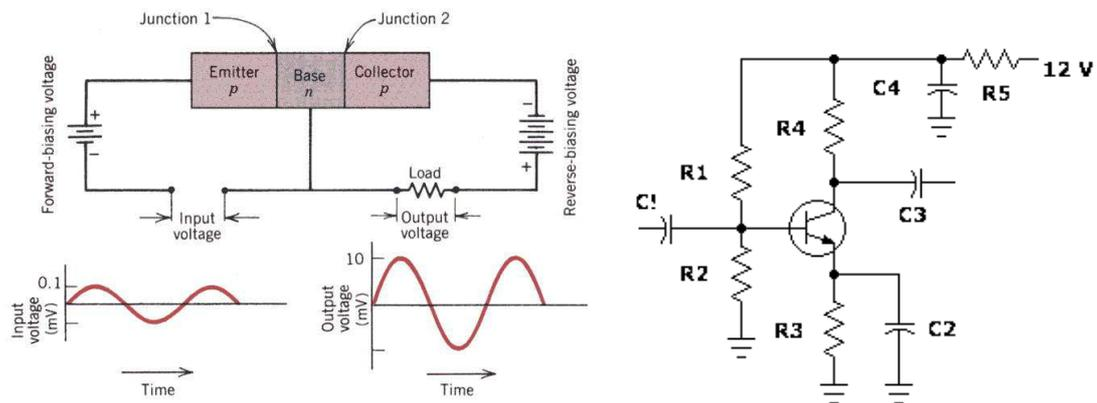
Figure 9. Left: Illustration of a pnp transistor and its use as an amplifier. Right: A transistor in a real amplifier circuit.
