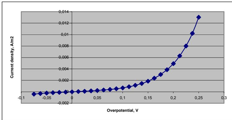
Figure 24. Current density vs overpotential for a system with  $i_0=0.0001 \text{ A/m}^2$ ,  $n=1$ ,  $\alpha_a = \alpha_c = 0.5$ ,  $T=298 \text{ K}$
