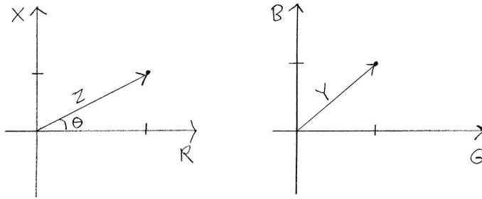
Figure 15. Representation of complex impedance (left) and complex admittance (right) in Cartesian coordinates.
