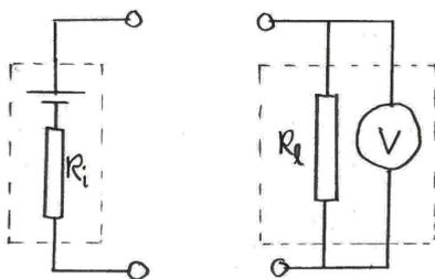
Figure 10. Schematic illustration of the internal resistance  $R_i$  of a DC voltage source (generally any generator, transistor, battery, fuel cell, etc.) and the input load resistance  $R_i$  of an input stage (e.g. voltmeter, amplifier).
