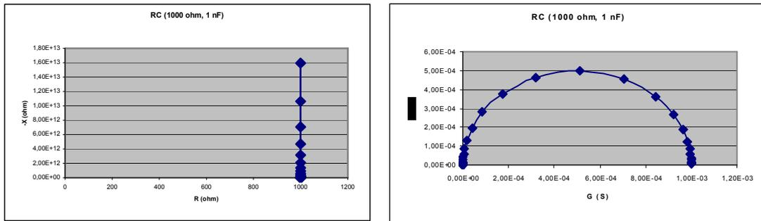
Figure 27. Nyquist-type impedance and admittance plots of a series circuit of one resistor and one capacitor, over a frequency range of  $10^{-5}$  to  $3 \cdot 10^7$  Hz (the range of a Solartron 1260). The impedance plot has  $-X$  as the  $y$ -axis according to common practice to get capacitive elements appear in the 1<sup>st</sup> quadrant.
