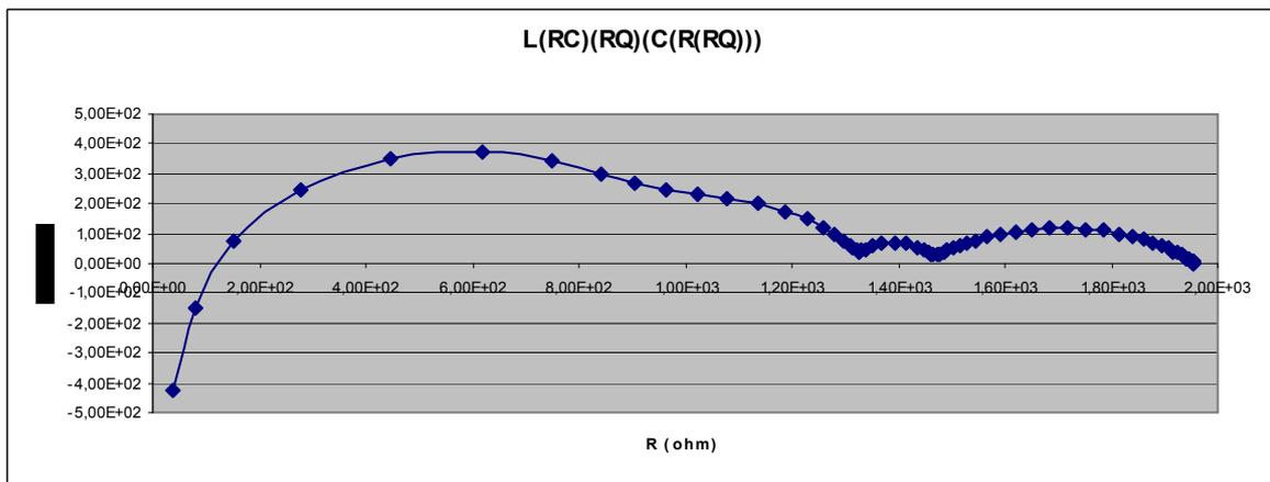
Figure 36. Nyquist impedance plot for a typical ceramic sample.
